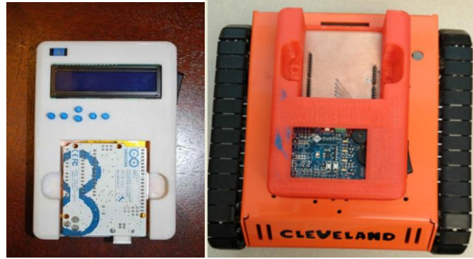
Figure 4 (a and b): RF-LCD Transmitter and RF-robot
